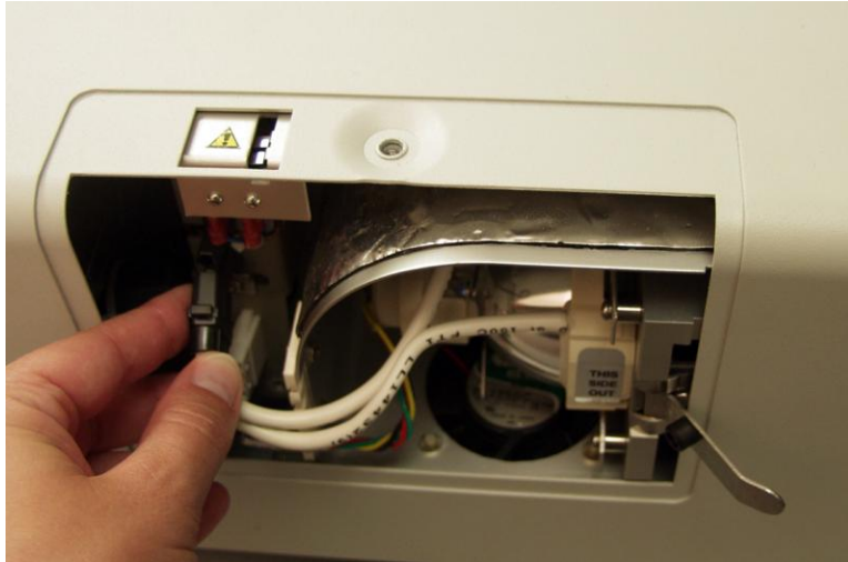
Figure 7 Lamp Power Connection
