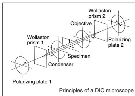
When the light from the light source passes through polarizing plate 1 (the polarizer), it will be polarized (changed to light that vibrates in one direction only). When this polarized light passes through Wollaston prism 1, it is split into two rays that have mutually perpendicular planes of polarization (direction of vibration); the two rays travel at a slight distance from each other.
