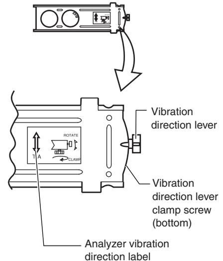
This figure is an illustration of the T-A DIC analyzer. For an illustration of the T-A-E motorized DIC analyzer, please refer to the instruction manual supplied with the T-HUBC HUB controller.
