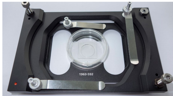
Figure 2 – ZEISS level-adjustable piezo stage insert
