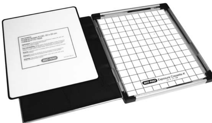
Fig. 2.2. Sample exposure cassette and phosphor screen.
