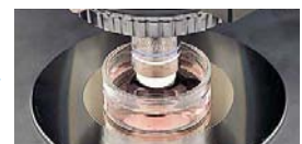
Long working distance, non-cover glass water immersion objective
